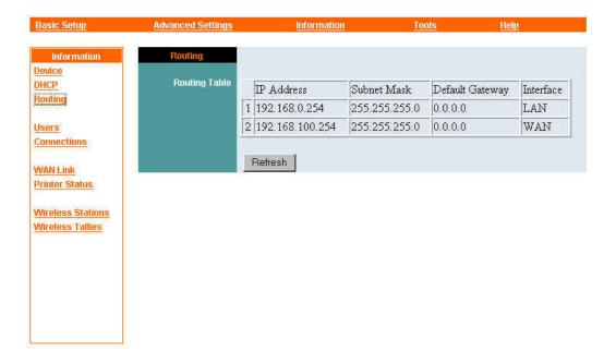
A learned or static route consists of a network address and subnet mask, the IP address of the gateway to that network, and the Wireless Gateway interface (LAN or WAN) through which that gateway can be reached.
